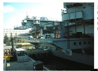
In the picture above, the superstructure called the "Island" is visible on the right. The control of flight operations and navigation of the ship is carried out from the island and a tour of those spaces was our next objective.
