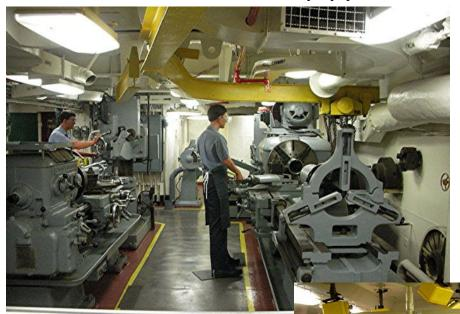
crew working in an extensive machine shop. Shown on the left is a display of the several industrial scale lathes and milling machines in the ship's machine shop with manikins in place.
